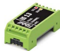
#13 Four-channel -10...+10V ADC
