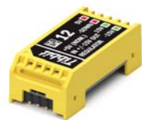
#12 Power regulator 5V→+15V/-15V
