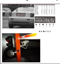
License plate recognition system (optional) scans, detects and performs the character recognition on the license plate number, supported by a camera system, suitable for proper license plate recognition day and night. It automatically forwards the license plate data and pictures for data storage and processing. This way the arrival and exit time of the truck is registered, plus the truck can be called by license plate number.
