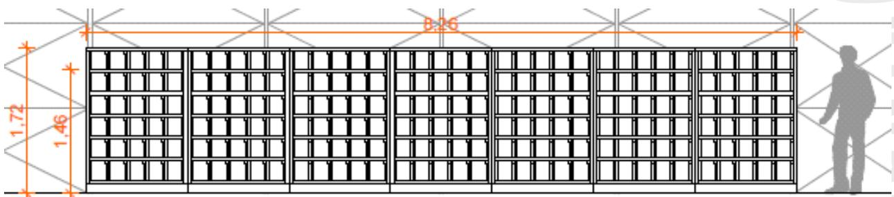
The AutoSafe210 string made with 7 cabinets and 210 doors. Each cabinet of the 7 has the same size, features with separate, built-in power supply and Ethernet Port. The 7 cabinets connect to the network with an 8 port Ethernet Switch.
