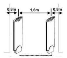
Two UltraPost detectors, gates are to be placed for one exit (e.g. 1,8m).
