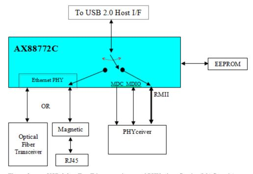
Figure 3 : USB 2.0 to Fast Ethernet and external PHYceiver Combo (MAC mode)
