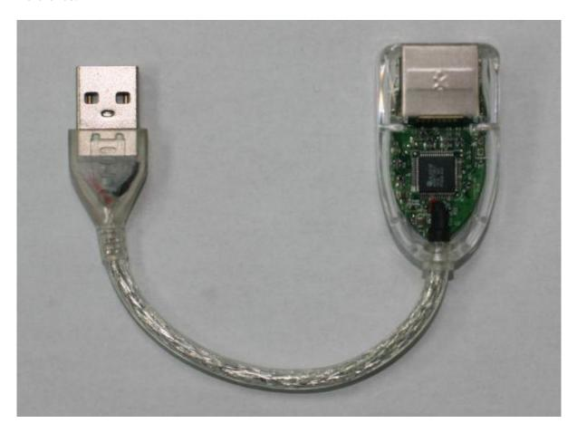
Figure 7. AX88772C USB to 100Base-TX Ethernet Demo Board
