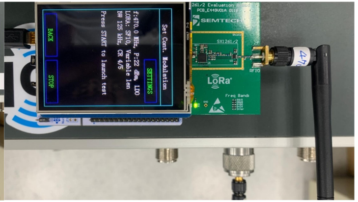
SX126 test via radiation connection
