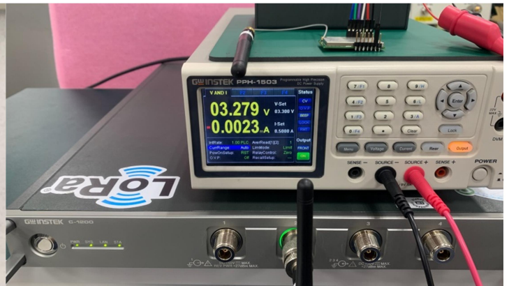
The DUT is controlled by C-1201 directly via UART, and PPH-1503 supplies DC power and measures the current consumption simultaneously
