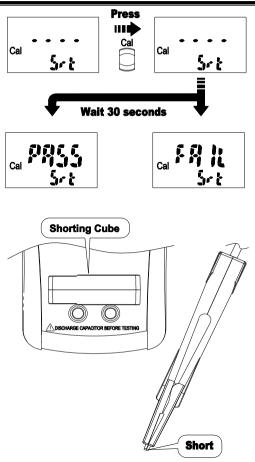
When "Srt" appears on the sub display, short the terminals or the SMD test probe, and then press the CAL button to start the short calibration. About 30 seconds later, the result of the short calibration appears on the main display. If the result is "pass", press the CAL button to complete the calibration. If the result is "fail", press the CAL button to exit the function.
