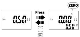
The Zero mode records the current input value as a reference and displays the reference on the sub display. Any inputs after this will be subtracted from the reference value and displayed on the main display. To use the Zero mode, follow the steps below.
