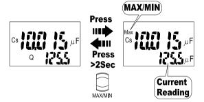
The MAX/MIN mode records the maximum and the minimum input values. When the inputs go below the recorded minimum value or above the recorded maximum value, the meter beeps and records the new value.
