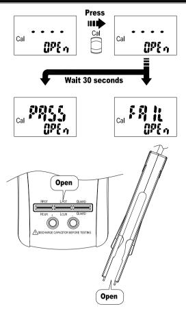
When "OPEn" appears on the sub display, make the terminal or the SMD test probe open, and press the CAL button to start the open calibration. About 30 seconds later, the result of the open calibration appears on the main display. If the result is "pass", press the CAL button to proceed to the next step. If the result is "fail", press the CAL button to exit the function. GUINSTEK LCR-914/915/916 User Manual
