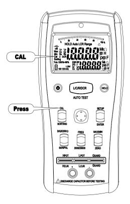
In order to achieve the best measurement results, calibration is essential. To calibrate the meter, press the CAL button.
