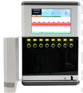
The intelligent modules containing eight key positions are connected to an RS485 network inside the cabinet. This network is connected via Ethernet to the cabinet's management software running on external PC. The RFID reader, the other storage units, the cabinet door locks and the door state sensors are also connected to the same RS485 network.
