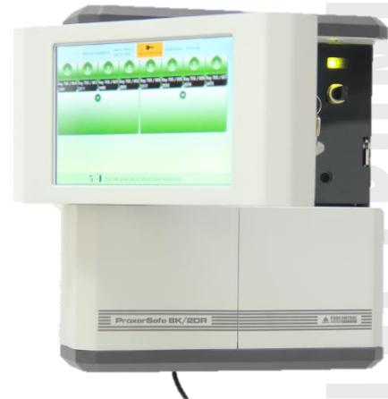
The intelligent modules containing eight key positions are connected to an RS485 network inside the cabinet. This network is connected via Ethernet to the cabinet's management software running on external PC. The RFID reader, the other storage units, the cabinet door locks and the door state sensors are also connected to the same RS485 network.
