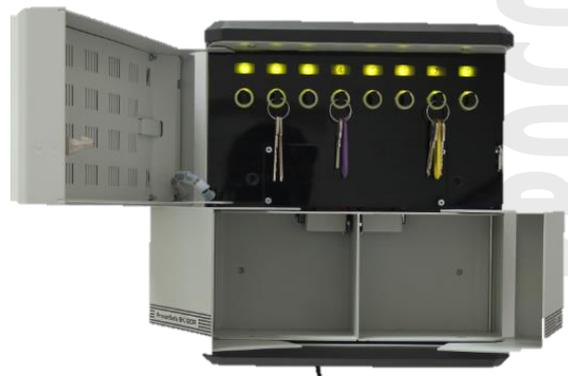
The device checks by default if the key has been put back to its original position. Keys switched are indicated, but the system allows putting the key into another slot, and logs the event. Sound signal can be turned on to indicate when keys are put back not in the right position. Key position identification function can be switched off, but it enables “Find the key” function.
