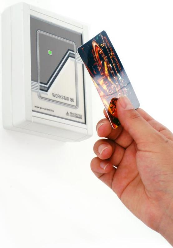
Access control and time-attendance terminal with one or two built-in RFID PROXIMITY (proximity) card-reader and sound signaller.
