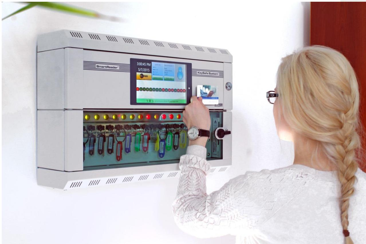
The KeySafe Lock is a safety key-storage cabinet, that can be opened only with personal RFID proximity card (transponder) or/and with a PIN code, optionally using fingerprint identification, if the device is a KeySafeLockBio. The offline type has an inbuilt computer. It is possible to connect it to a computer network and to check remotely who and when took which key and for how long time.
