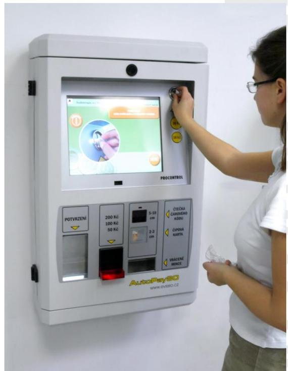
Beyond the key, an RFID card is also required for opening the automat. It contains the identification code of the responsible person (cashier). This code and the name of the responsible person are included in an encrypted way on the digitally stored master sheet of the automat. (At the request of the owner more key cards can be issued and programmed.)
