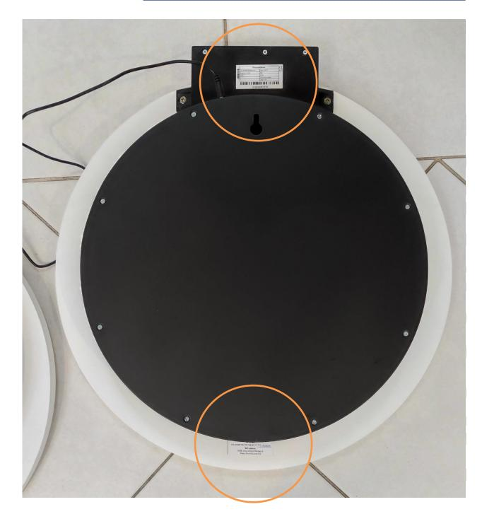
For service purposes, it may be necessary to inform the service about the serial number of the clock: you can find the 12-digit serial number on the sticker at the top of the back of the clock.
