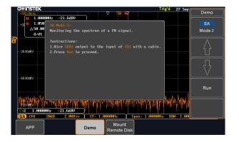
This carrier waveform of FM is sine 15MHz, 500mVpp; FM frequency is 50kHz; Frequency deviation is 5MHz. Now, we could clearly observe the data of frequency domain signal (approximately 10MHz) from cursor's markers.
