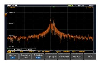
4. Select SA mode 4 and RUN, the screen will display linear frequency sweep in the frequency domain.
