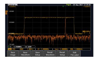
With the above 4 signal demonstrations we can clearly understand the frequency domain analysis capability of MDO-2000E. MDO-2000E standardly provides a 25MHz AWG, which can be collocated with this demo APP to allow beginners to quickly learn and show the operation of spectrum analyzer without preparing other signal generators or DUTs. Settings include start, stop, span frequency, spectrum traces, and RBW etc.
